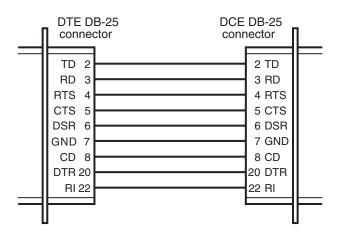
Figure F-1. 25-pin to 25-pin RS-232 cable.
